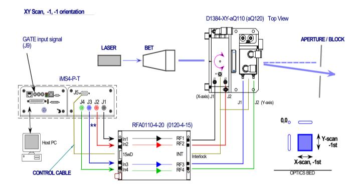
Figure 4: Typical Connection Configuration
