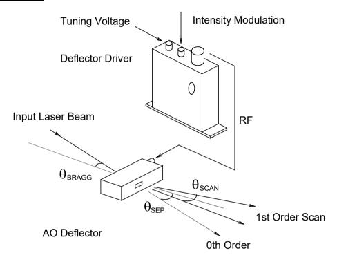
The input Bragg angle, relative to a normal to the optical surface and in the plane of deflection is :
