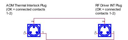
The interlock signal must be connected. Contacts closed for normal operation.
