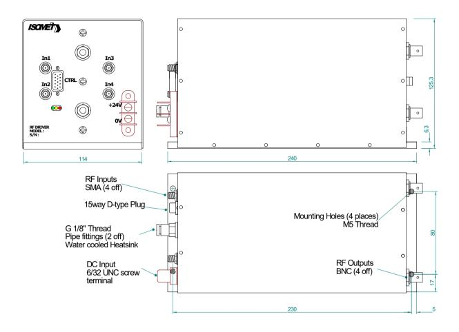
Figure 1: Driver Installation
